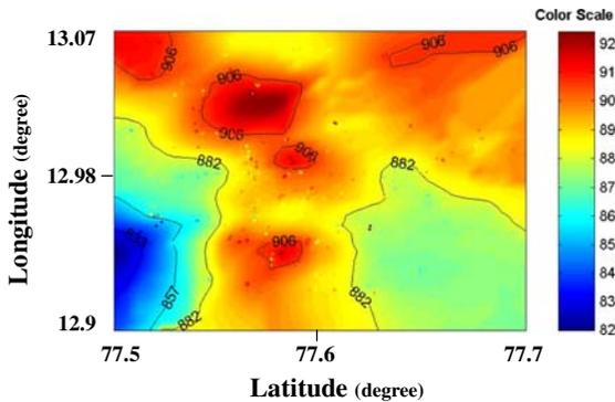
**Fig. 21** Surface of reduced level of rock depth using Ordinary Kriging
