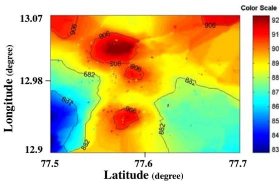
**Fig. 22** Surface of reduced level of rock depth using ANN
