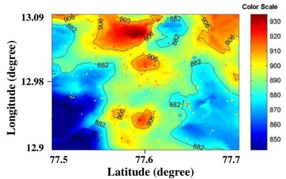
**Fig. 23** Surface of reduced level of rock depth using SVM
